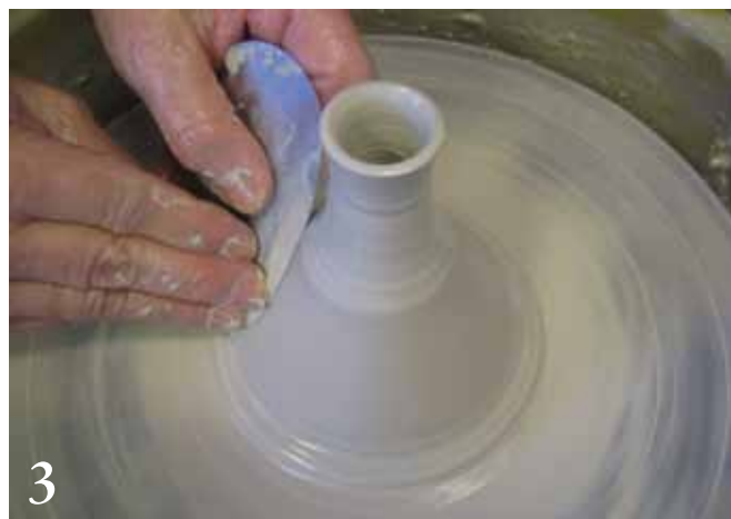
3 When you've finished throwing the spout, use a rib to smooth and compress the surface.
