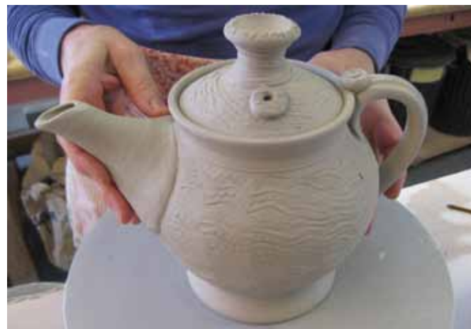
12 Finished greenware pot. Cover the finished piece loosely with plastic and allow the moisture to equalize for a couple of days.
