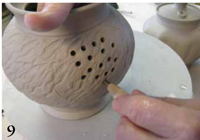
9 Create strainer holes within the outline of the wide end of the spout.
