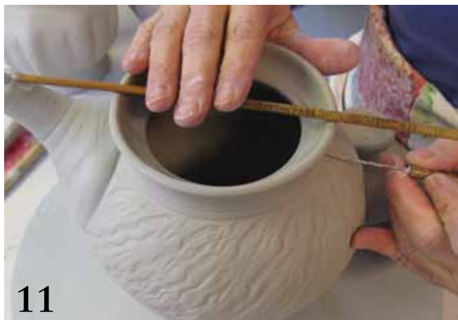
11 Lay a straight edge across the teapot extending from the tip of the spout and across the opening to determine the handle placement.
